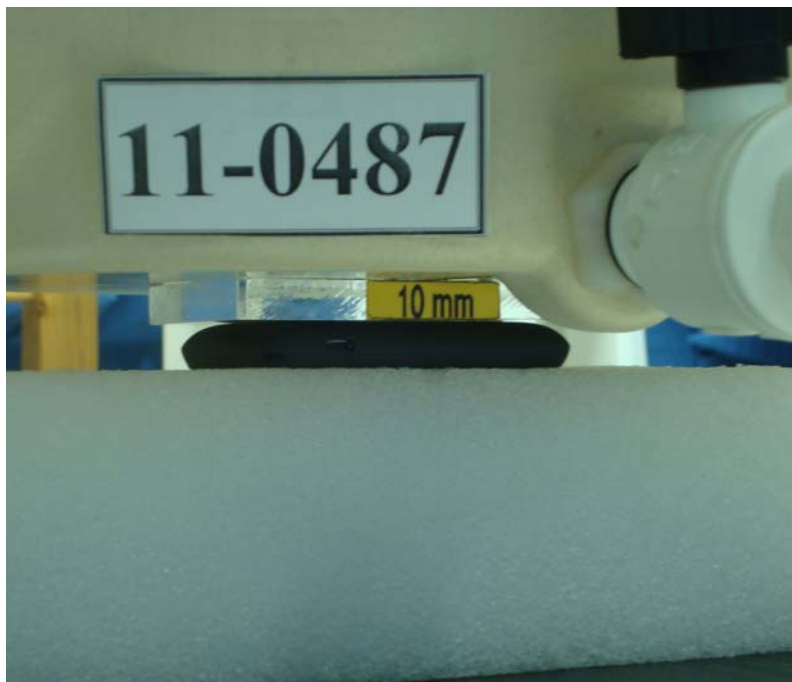
Figure 6. Body SAR Test Setup (Flat Section)
