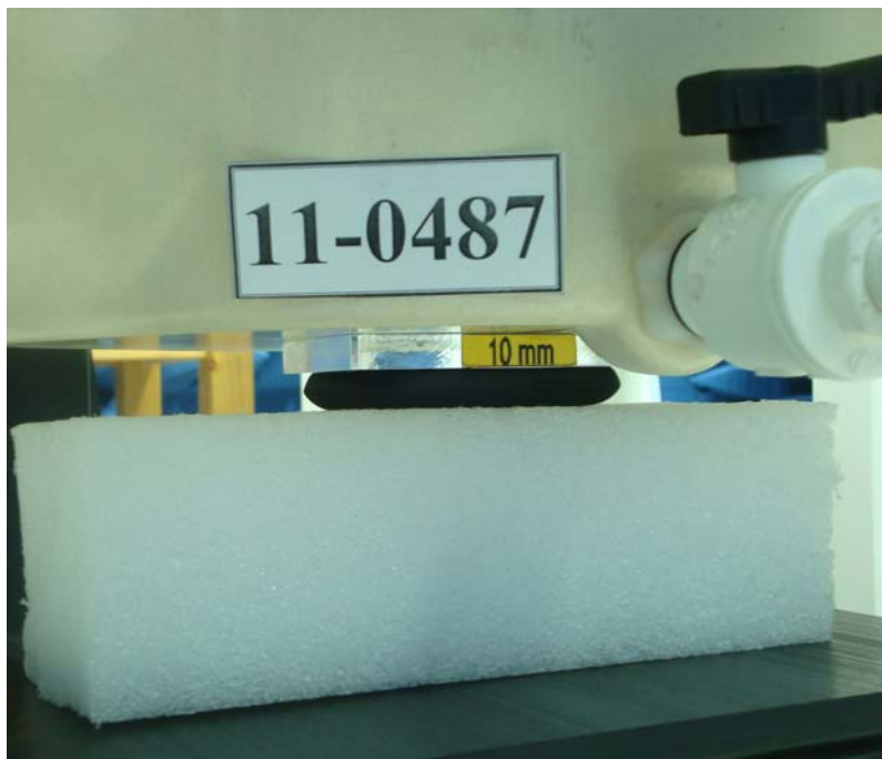
Figure 5. Body SAR Test Setup (Flat Section)
