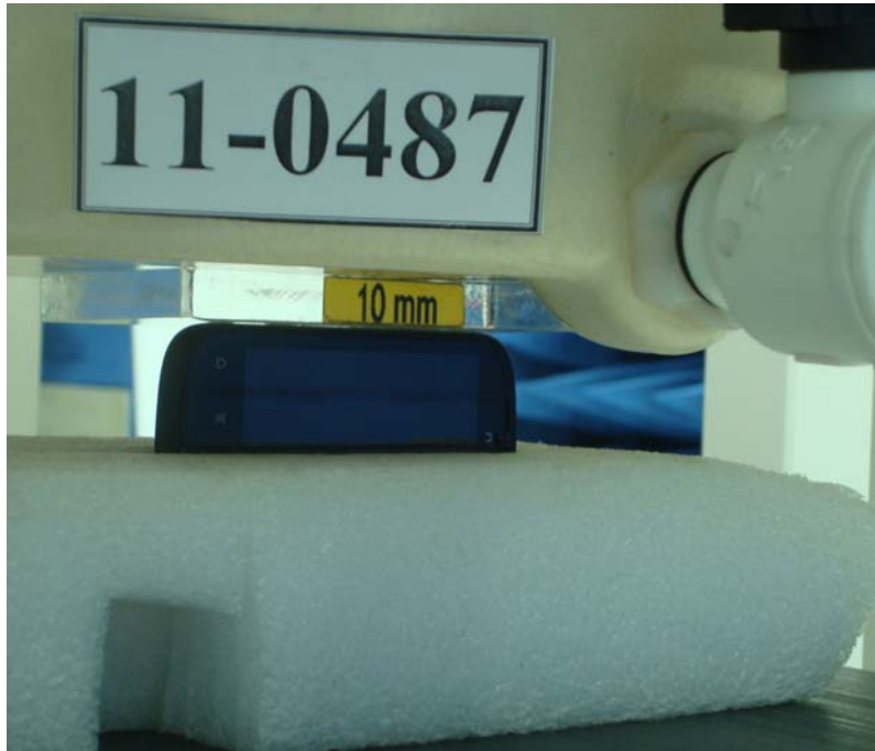
Figure 7. Body SAR Test Setup (Flat Section)
