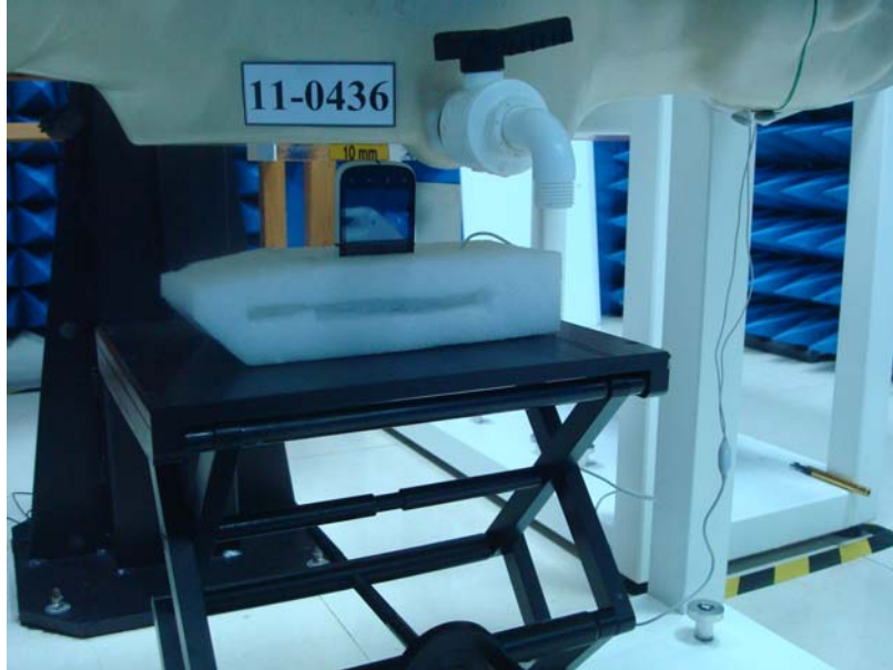
Figure 9. Body SAR Test Setup (Flat Section)
