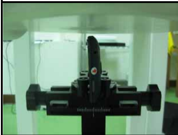
LEFT SIDE WITH 1 CM GAP (DUT WITHOUT EARPHONE)
