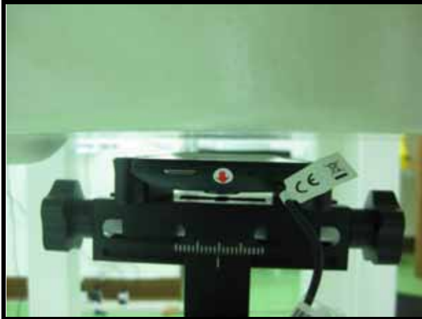
FRONT FACE WITH 1 CM GAP (DUT WITH EARPHONE)
