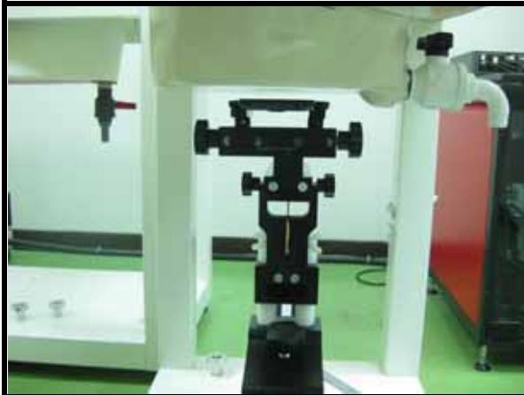
Front Face with 1 cm Gap (DUT without Earphone)
