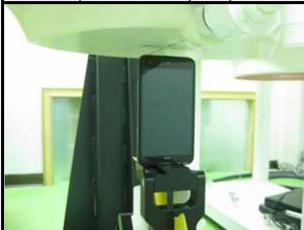
Down Edge with 1 cm Gap (DUT without Earphone)
