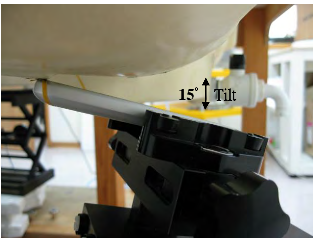
Fig.4 Right Head Section / Ear-Tilt Position(15°)
