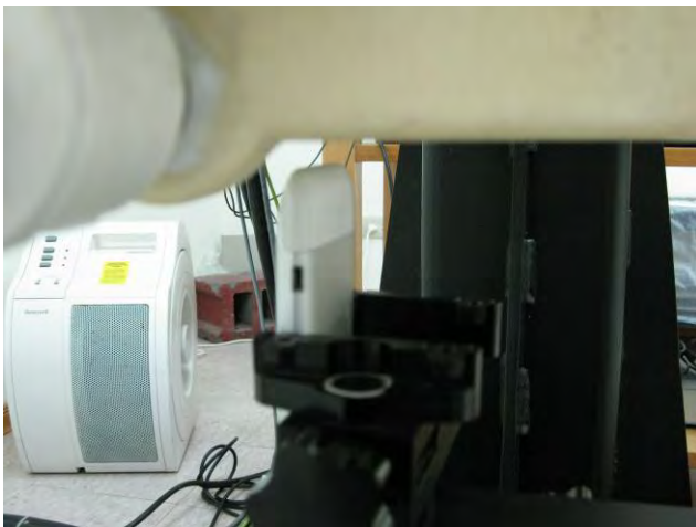
Fig.9 Hotspot mode- EUT Bottom to flat phantom and distance between flat phantom and mobile phone is 1 cm.
