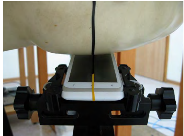
Fig.6 Left Head Section / Ear-Tilt Position(15°)
