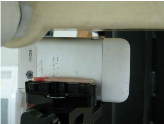
Fig.11 Hotspot mode- EUT Left to flat phantom and distance between flat phantom and mobile phone is 1 cm.
