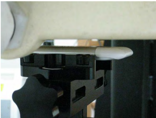
Fig.8 Hotspot mode- EUT back to flat phantom and distance between flat phantom and mobile phone is 1 cm.
