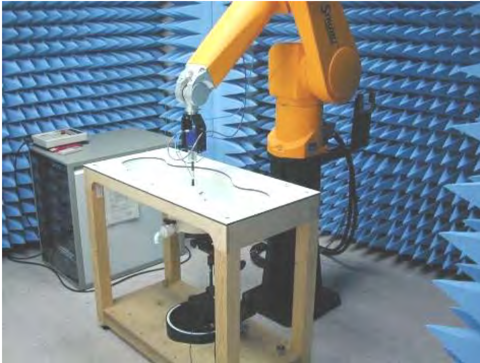
Fig.1 Photograph of the SAR measurement System
