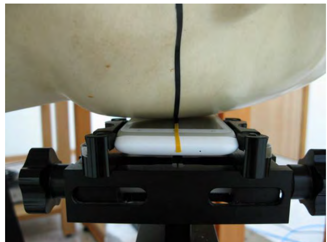
Fig.5 Left Head Section / Cheek-Touch Position
