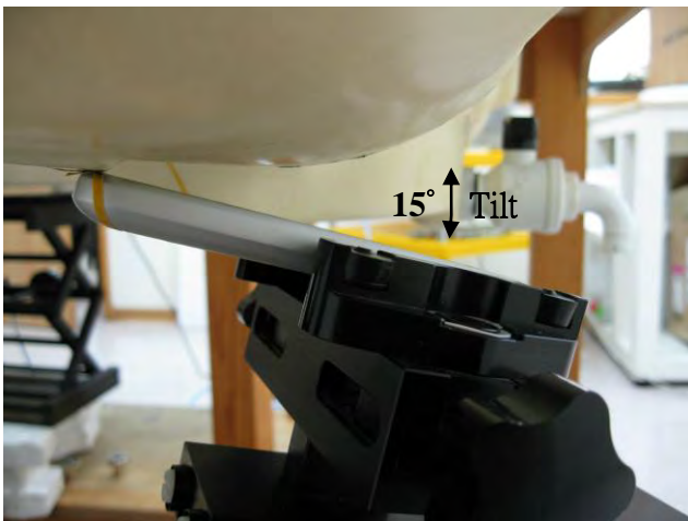
Fig.4 Right Head Section / Ear-Tilt Position(15°)
