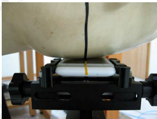
Fig.5 Left Head Section / Cheek-Touch Position
