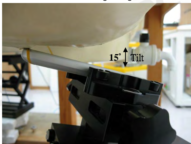
Fig.4 Right Head Section / Ear-Tilt Position(15°)
