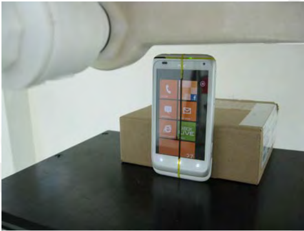
Fig.9 Hotspot mode- EUT Top to flat phantom and distance between flat phantom and mobile phone is 1 cm.
