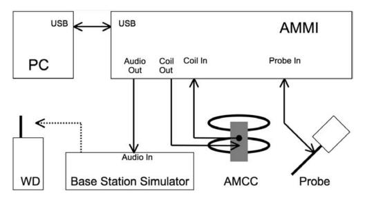
Figure 5.1: T-Coil setup cabling
