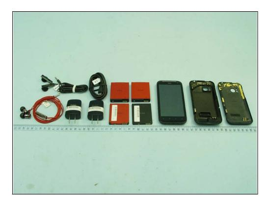
The EUT were powered by the following adapters, battery & accessories:
