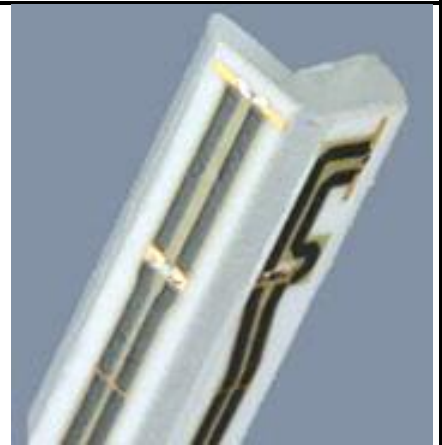
Fig 5.2 Photo of E-field Probe
