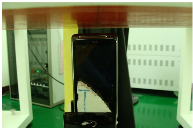
Top Side of the DUT with Phantom 1 cm Gap for DUT without Earphone
