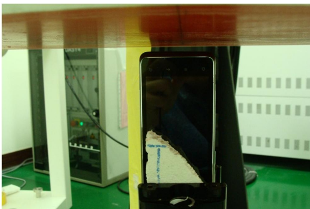
Bottom Side of the DUT with Phantom 1 cm Gap for DUT without Earphone
