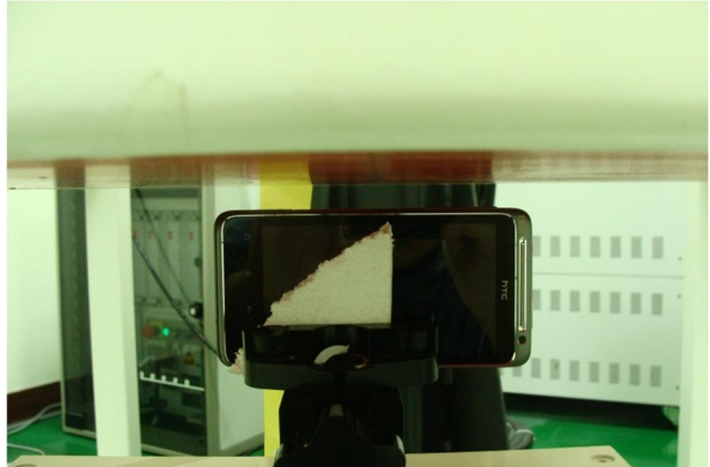
Left Side of the DUT with Phantom 1 cm Gap for DUT without Earphone
