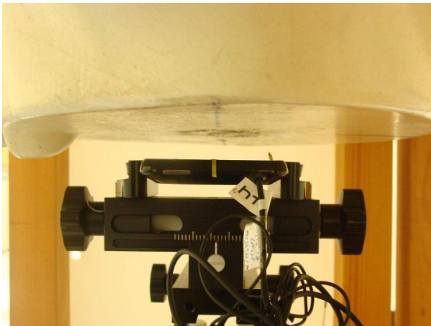
Front of the DUT with Phantom 1 cm Gap for DUT with Earphone 3
