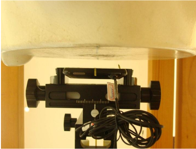
Front of the DUT with Phantom 1 cm Gap for DUT with Earphone 1
