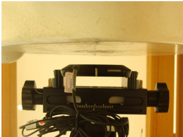
Back of the DUT with Phantom 1 cm Gap for DUT with Earphone 1
