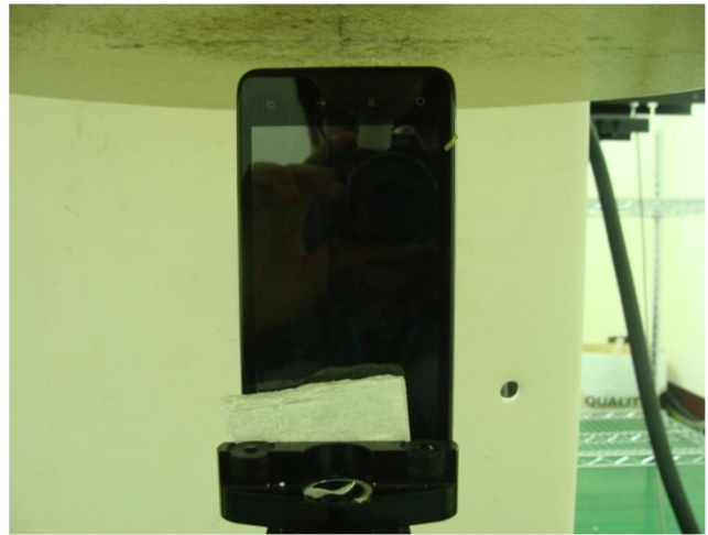
Down Side of the DUT with Phantom 1 cm Gap for DUT without Earphone
