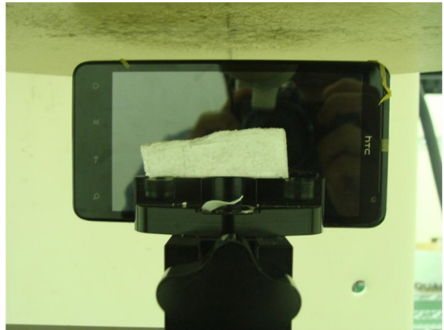
Left Side of the DUT with Phantom 1 cm Gap for DUT without Earphone
