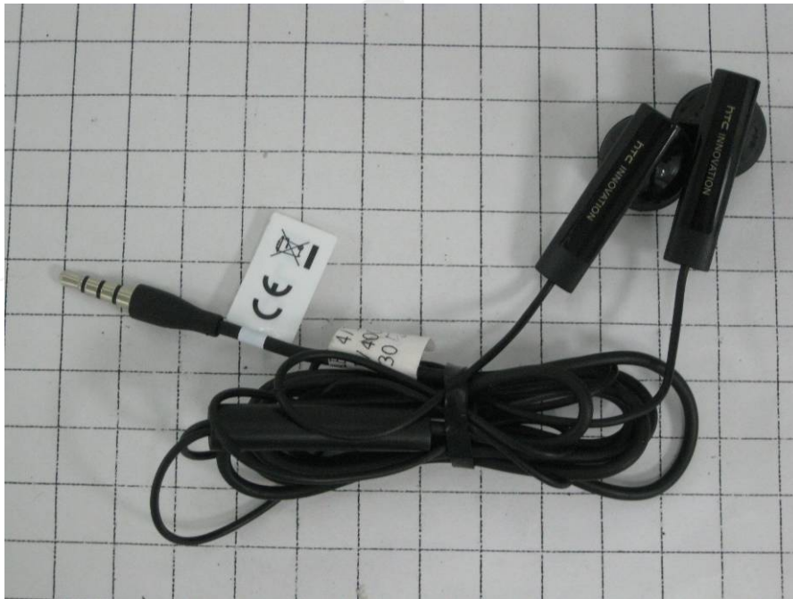
Fig.23 Headset (Supplier name : Foster Model name : RC E160 )
