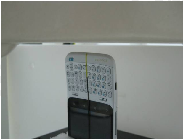
Fig.10 Body worn- EUT Bottom to flat phantom and distance between flat phantom and mobile phone is 1 cm.
