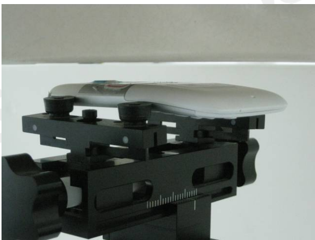
Fig.8 Body worn- EUT back to flat phantom and distance between flat phantom and mobile phone is 1 cm.
