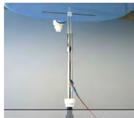
Photograph of the dipole Antenna
