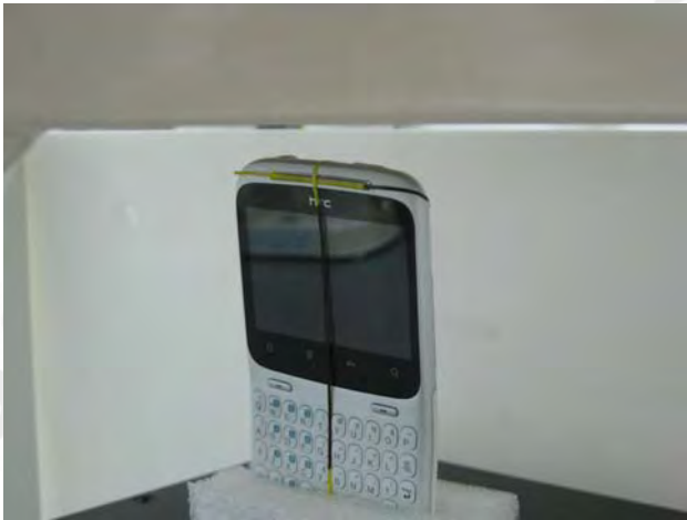
Fig.9 Body worn- EUT Top to flat phantom and distance between flat phantom and mobile phone is 1 cm.
