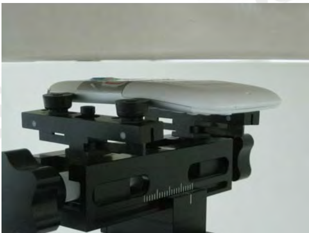
Fig.8 Body worn- EUT back to flat phantom and distance between flat phantom and mobile phone is 1 cm.
