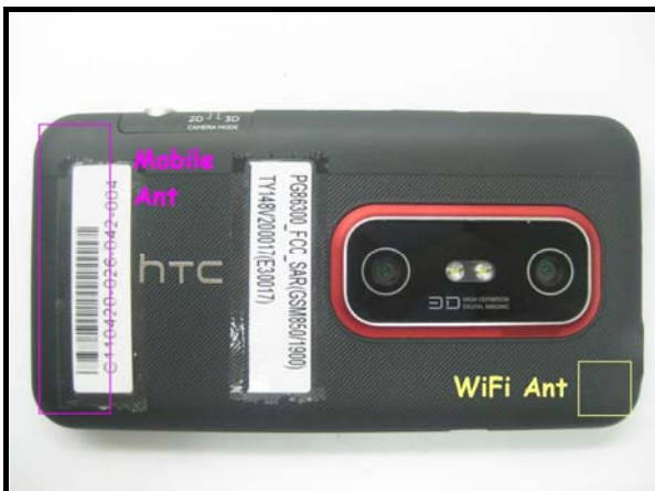
DESCRIPTION OF ANTENNA LOCATION
