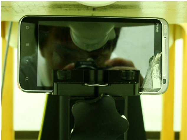
Left Side of the DUT with Phantom 1.0 cm Gap for DUT without Earphone
