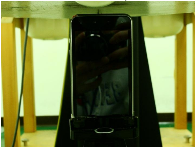
Bottom Side of the DUT with Phantom 1.0 cm Gap for DUT without Earphone
