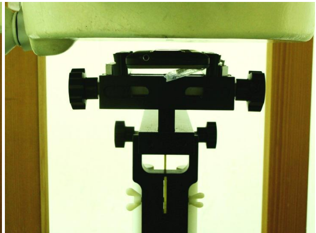
Rear Face of the DUT with Phantom 1.0 cm Gap for DUT without Earphone
