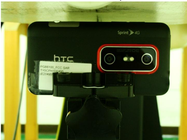
Right Side of the DUT with Phantom 1.0 cm Gap for DUT without Earphone
