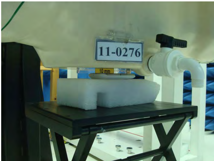
Figure 5. Body SAR Test Setup (Flat Section)
