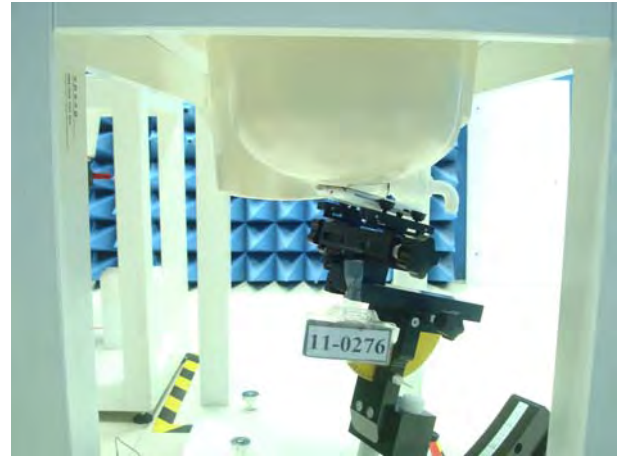
Figure 2. Right Head SAR Test Setup (Tilted)
