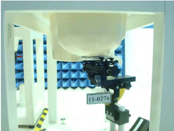
Figure 1. Right Head SAR Test Setup (Cheek)
