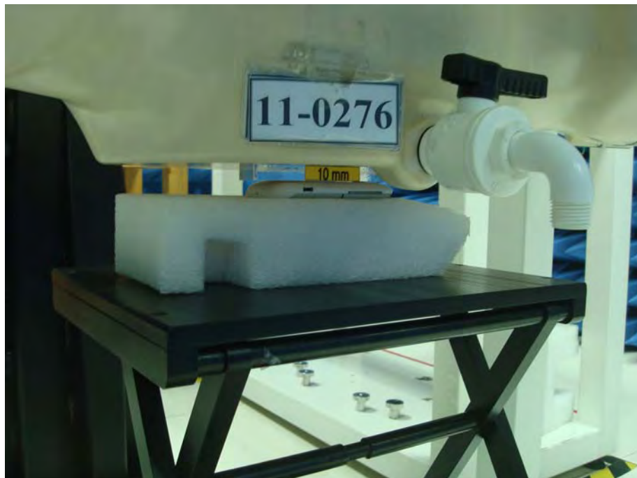
Figure 6. Body SAR Test Setup (Flat Section)
