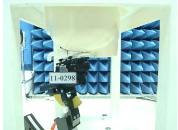
Figure 4. Left Head SAR Test Setup (Tilted)
