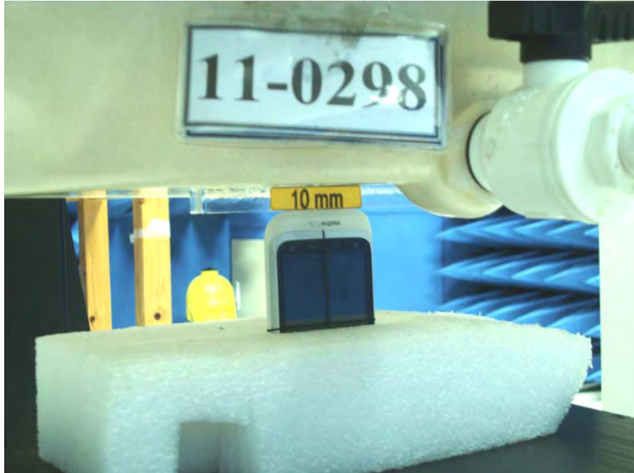
Figure 11. Body SAR Test Setup (Flat Section)
