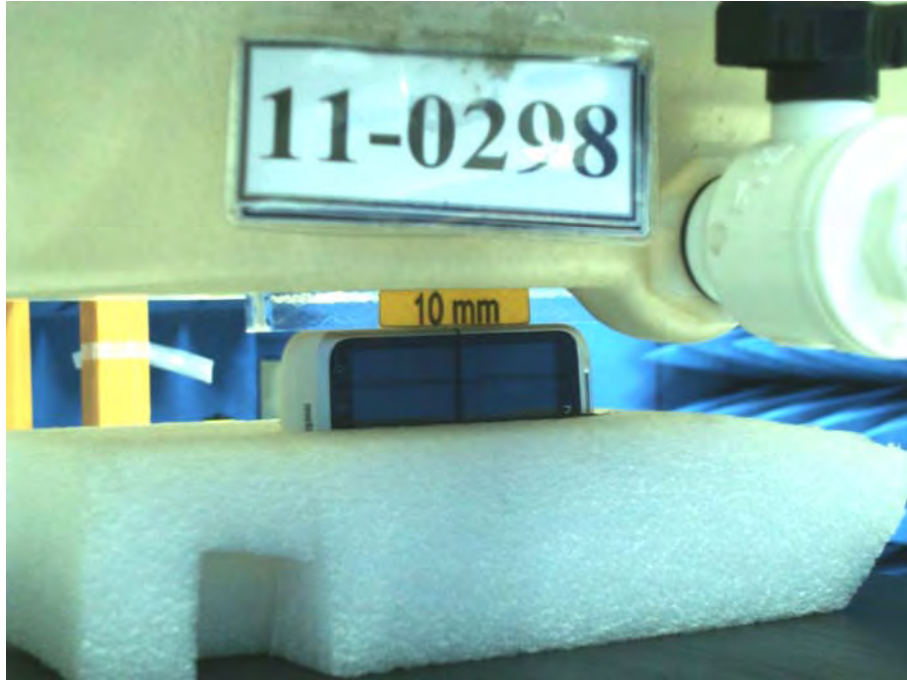
Figure 9. Body SAR Test Setup (Flat Section)
