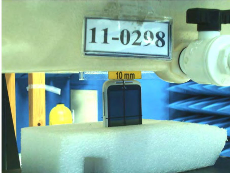
Figure 12. Body SAR Test Setup (Flat Section)
