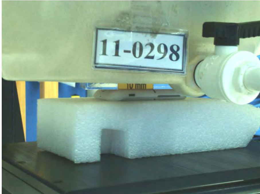
Figure 8. Body SAR Test Setup (Flat Section)
