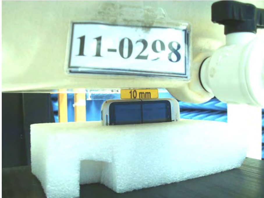
Figure 10. Body SAR Test Setup (Flat Section)
