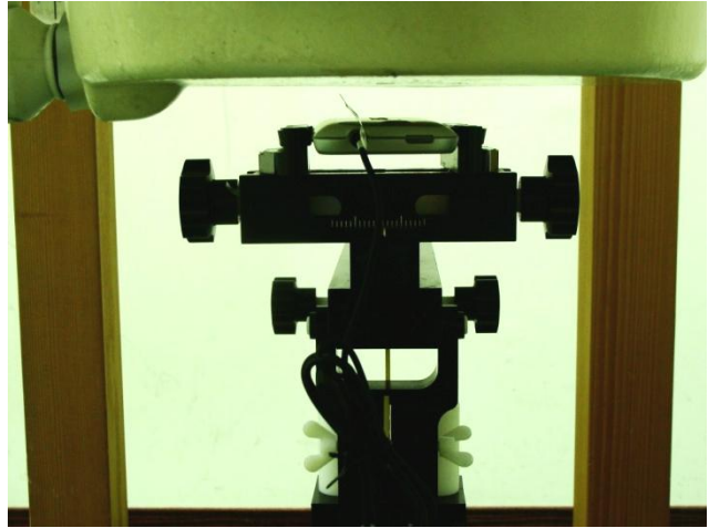
Rear Face of the DUT with Phantom 1 cm Gap (DUT with Earphone)
