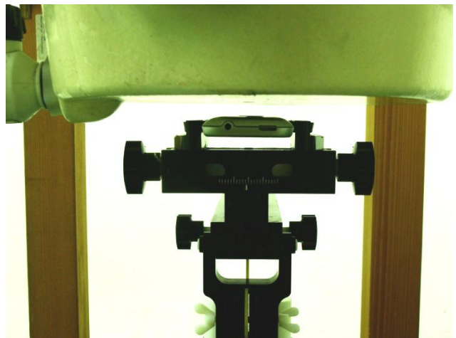
Rear Face of the DUT with Phantom 1 cm Gap (DUT without Earphone)
