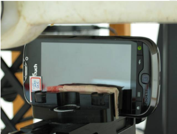
Fig.15 Hotspot mode - EUT Right to flat phantom and distance between flat phantom and mobile phone is 1 cm.
