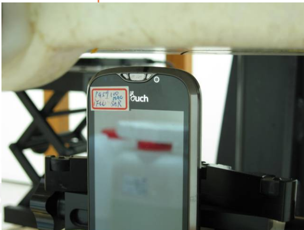
Fig.13 Hotspot mode - EUT Top to flat phantom and distance between flat phantom and mobile phone is 1 cm.
