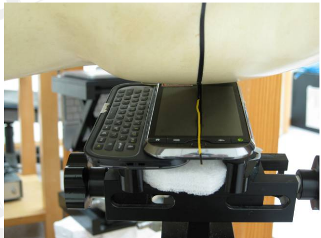
Fig.10 Left Head Section / Ear-Tilt Position(15°)_ Slider on
