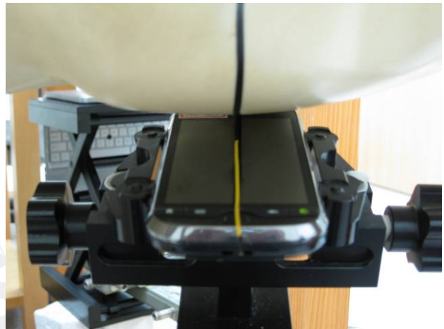
Fig.6 Left Head Section / Ear-Tilt Position(15°)_ Slider off
