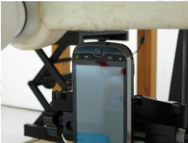
Fig.14 Hotspot mode - EUT Bottom to flat phantom and distance between flat phantom and mobile phone is 1 cm.
