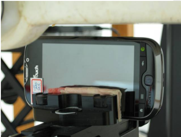
Fig.15 Hotspot mode - EUT Right to flat phantom and distance between flat phantom and mobile phone is 1 cm.
