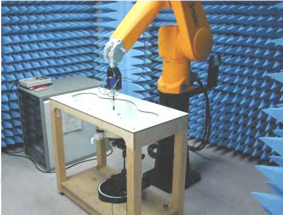
Fig.1 Photograph of the SAR measurement System
