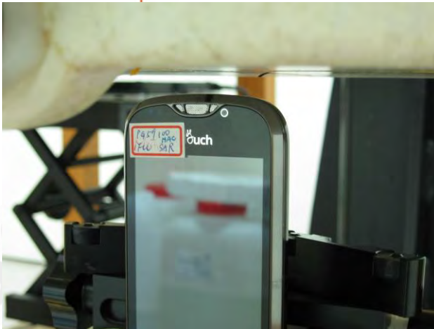
Fig.13 Body worn- EUT Top to flat phantom and distance between flat phantom and mobile phone is 1 cm.
