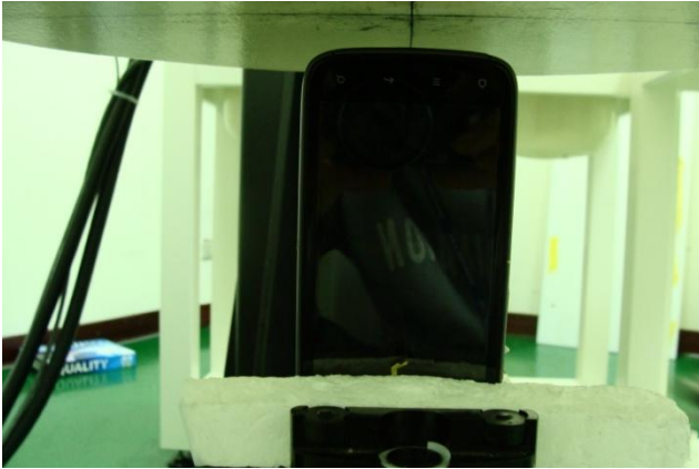
Bottom Side of the DUT with Phantom 1 cm Gap (DUT without Earphone)
