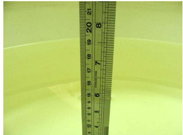
Fig 6.2 Photo of Liquid Height for Body SAR
