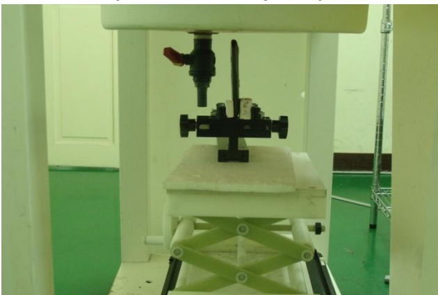
Top Side of the DUT with Phantom 1 cm Gap (DUT without Earphone)
