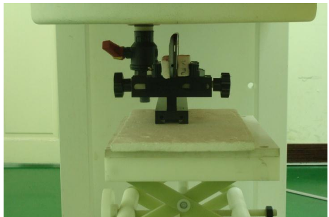
Right Side of the DUT with Phantom 1 cm Gap (DUT without Earphone)
