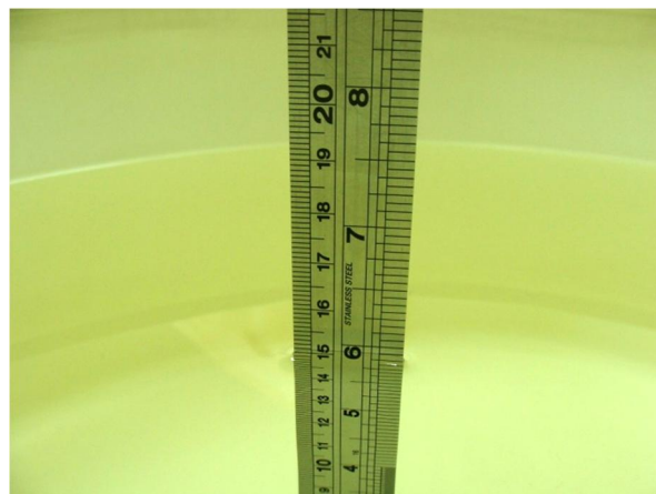
Fig 6.2 Photo of Liquid Height for Body SAR
