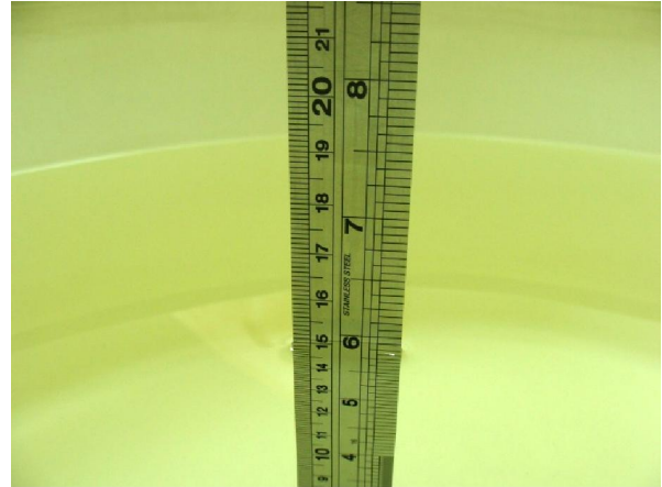
Fig 6.2 Photo of Liquid Height for Body SAR
