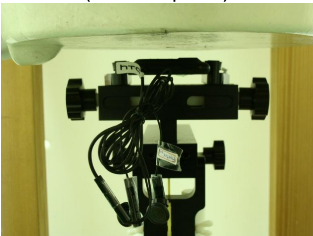
Rear Face of the DUT with Phantom 1 cm Gap (DUT with Earphone 3)
