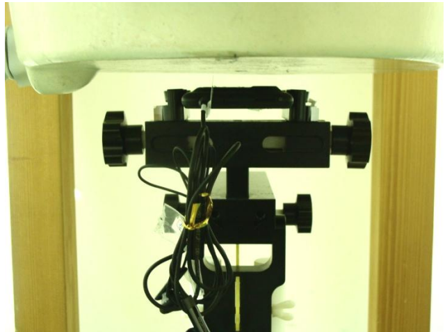
Rear Face of the DUT with Phantom 1 cm Gap (DUT with Earphone 2)
