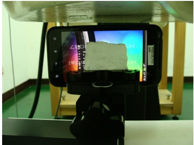
Left Side of the DUT with Phantom 1 cm Gap (DUT without Earphone)
