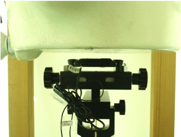
Rear Face of the DUT with Phantom 1 cm Gap (DUT with Earphone 1)
