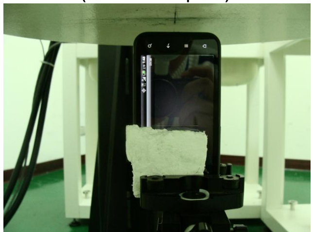
Bottom Side of the DUT with Earphone 1 cm Gap (DUT without Earphone)
