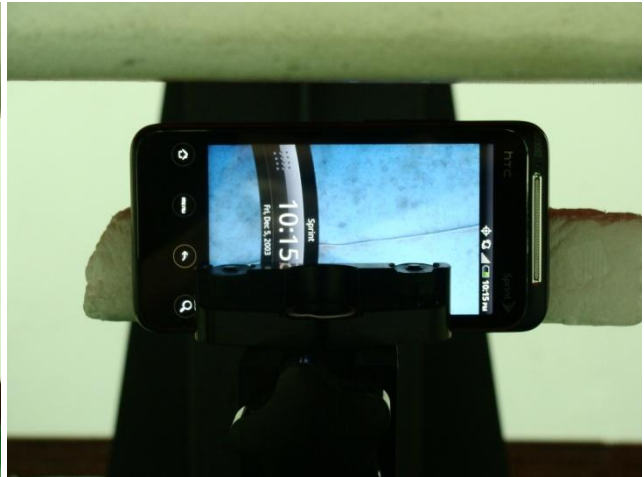
Left Side of the DUT with Phantom 1.0 cm Gap for DUT Slide Off Mode without Earphone
