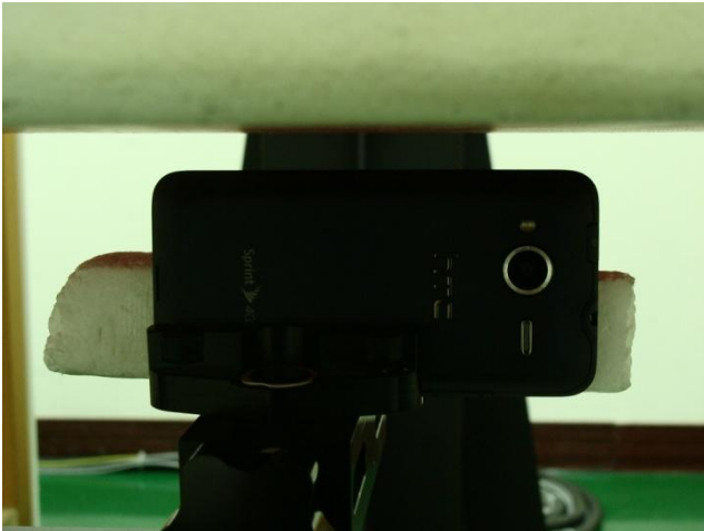
Right Side of the DUT with Phantom 1.0 cm Gap for DUT Slide Off Mode without Earphone
