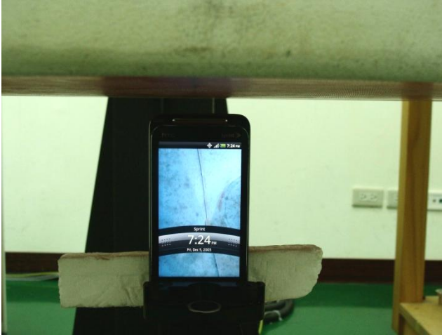
Top Side of the DUT with Phantom 1.0 cm Gap for DUT Slide Off Mode without Earphone
