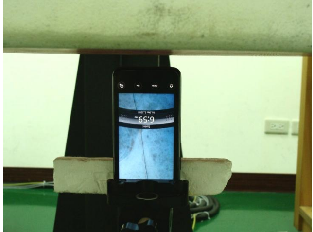
Bottom Side of the DUT with Phantom 1.0 cm Gap for DUT Slide Off Mode without Earphone
