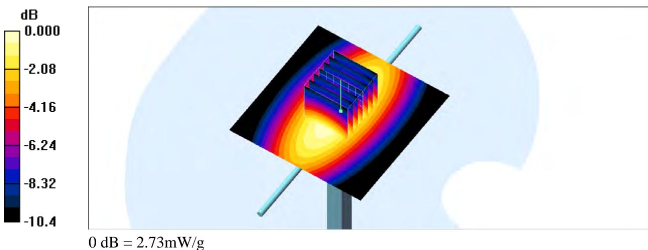
**System Check\_Head\_835MHz\_110301****DUT: Dipole 835 MHz**
