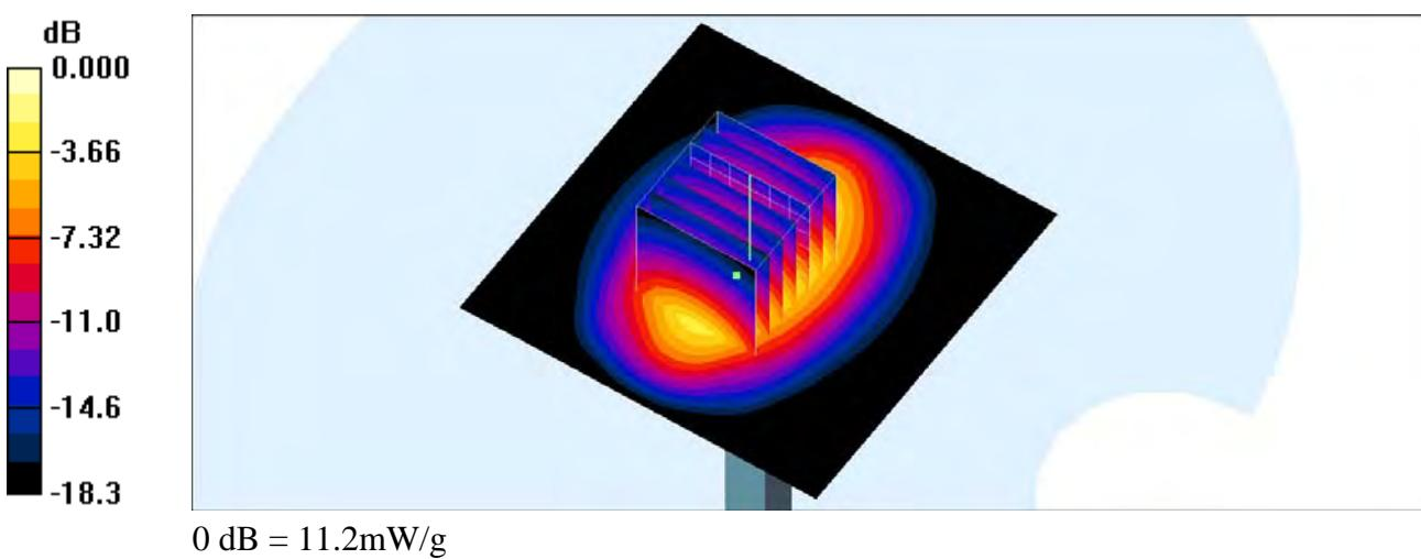
**System Check\_Head\_1900MHz\_110301****DUT: Dipole 1900 MHz**
