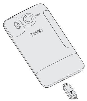
2. Plug in the power adapter to an electrical outlet to start charging the battery.
