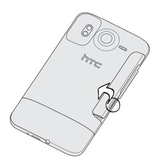
3. Pull the battery out from the battery compartment.
