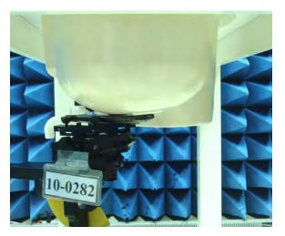
Figure 3. Left Head SAR Test Setup (Cheek)
