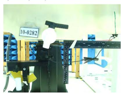
Figure 5. Body SAR Test Setup (Flat Section)
