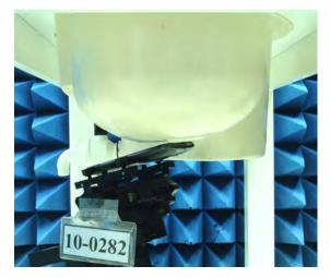
Figure 4. Left Head SAR Test Setup (Tilted)
