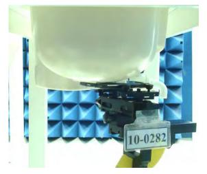
Figure 1. Right Head SAR Test Setup (Cheek)
