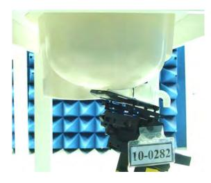
Figure 2. Right Head SAR Test Setup (Tilted)
