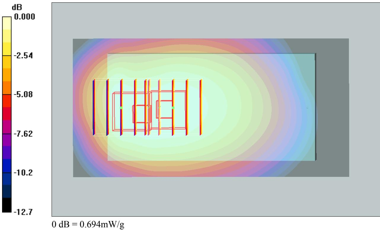
**#60 GSM850\_GPRS12\_Bottom\_1.5cm\_Ch128\_Battery 2\_Slide Off\_2D****DUT: 062328**
