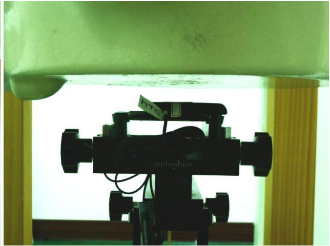
Bottom of the DUT with Phantom 1.5 cm Gap for Slide Left
