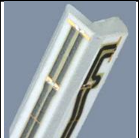
Fig 5.2 Photo of E-field Probe
