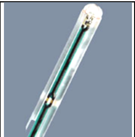
Fig 5.3 Photo of H-field Probe
