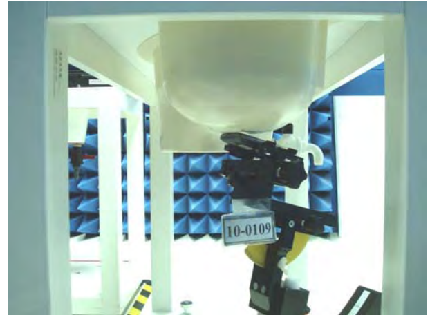
Figure 2. Right Head SAR Test Setup (Tilted)
