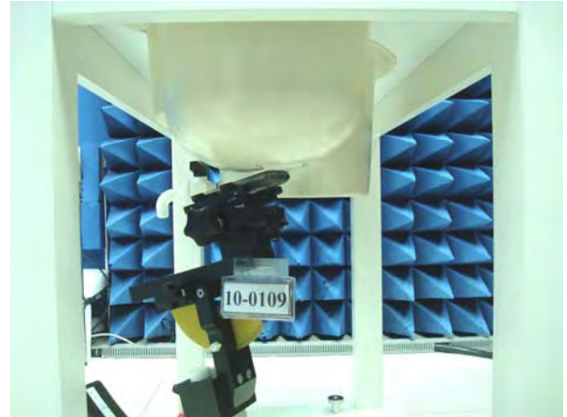
Figure 4. Left Head SAR Test Setup (Tilted)
