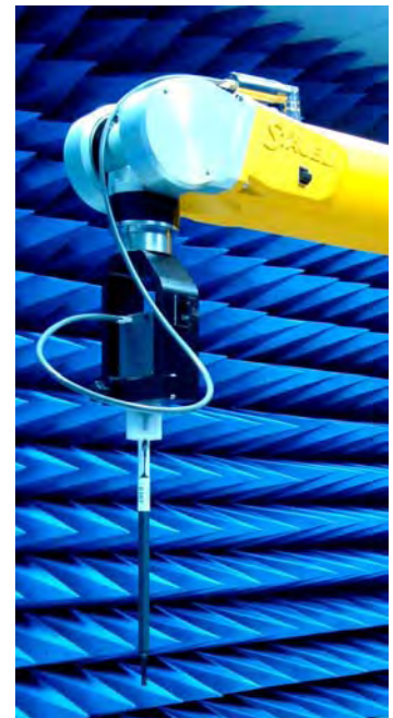
Figure 4. Probe setup on robot
