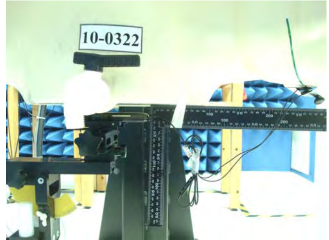
Figure 10. Body SAR Test Setup (Flat Section)_Close
