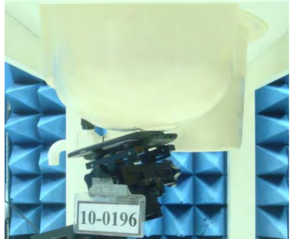
Figure 5. Left Head SAR Test Setup (Tilted) _Open
