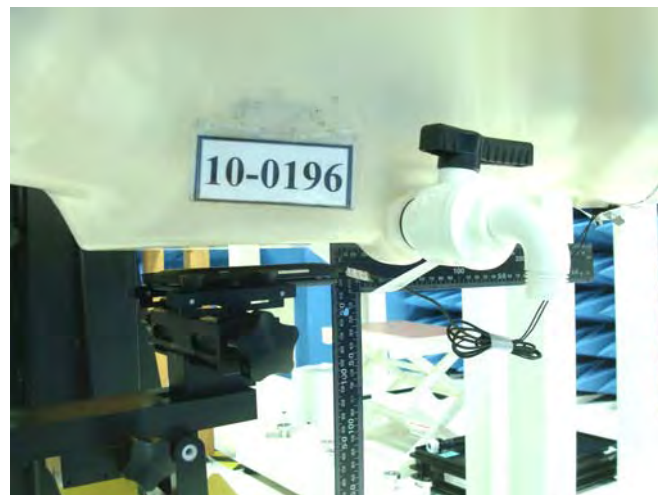
Figure 8. Body SAR Test Setup (Flat Section)_Close
